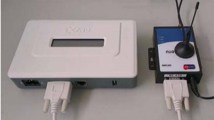
Host communication mode: in this mode, you can directly read data from the ECU. ECU use RS232 serial DB9 male interface, users through the corresponding female interface or extension cord to connect, also can use RS232 to RS485 interface converter.
